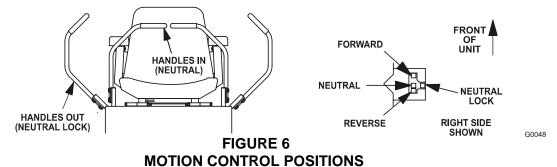
By moving both levers an *equal* amount forward or back from the neutral position the machine can be caused to move forward or backward in a straight line.
